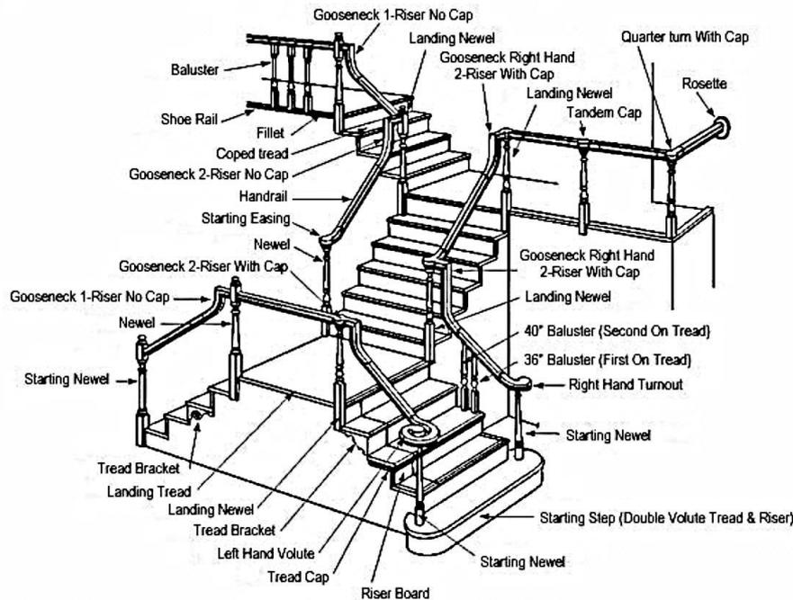
**BALUSTER** – A vertical member, used to fill the open area between the railing and the floor or tread, adding safety, support and stability to the balustrade.
