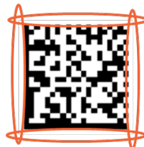
Figure 4-19 Example of the Data Matrix Quiet Zone
