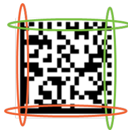
Figure 4-17 Example of the Data Matrix finder pattern
