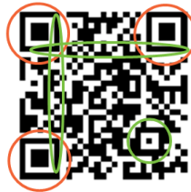
Figure 4-18 Example of the QR Code finder pattern
