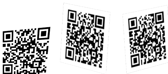
Figure 7-8 Examples of grid non-uniformity
